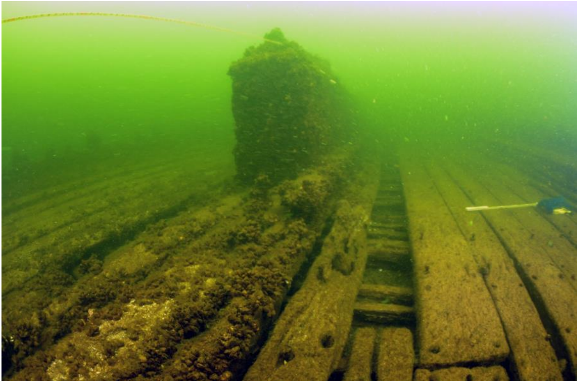
Figure 6. Aft end of the centerboard trunk, looking forward
