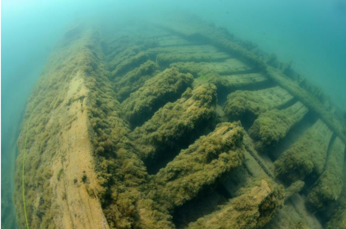
Figure 20. Keelson assembly and starboard side hull with reinforced framing
